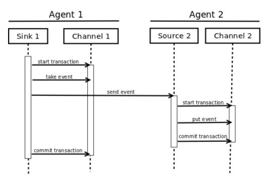
A Transaction is implemented within a Channel implementation. Each source and sink that is connected to a Channel must obtain a Transaction object. The sources use a Channel Processor to manage the Transactions, the sinks manage them explicitly via their configured Channel. The operation
