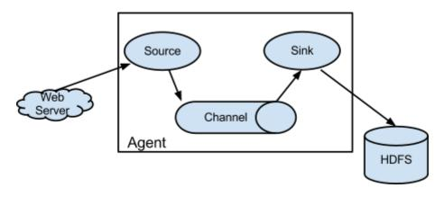
A source consumes Events having a specific format, and those Events are delivered to the source by an external source like a web server. For example, an Avrosource can be used to receive Avro Events from clients or from other Flume agents in the flow. When a source receives an Event, it stores it into one or more channels. The channel is a passive store that holds the Event until that Event is consumed by a
